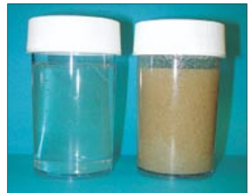
Proppant settling: 3% KCL with 6% VES and 8 PPA
