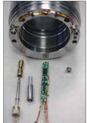
e Trigger ™ electronic controller replaces the MPas ™ box area with an electronic sub housing the programmable trigger assembly
